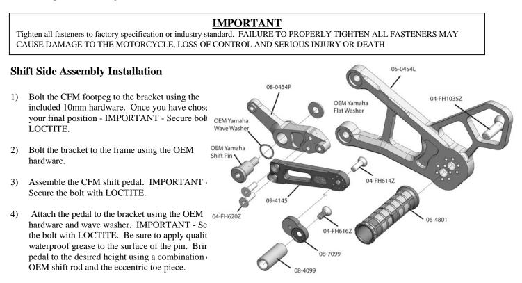
5) Attach the OEM heim joint to the pedal in your desired location (see picture at bottom for standard or GP shift). The heim joint threads into the pedal from the outside using the OEM bolt. IMPORTANT - Secure all bolts with LOCTITE.
